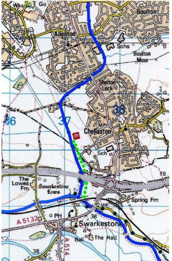
The blue line running north shows the original route and the green dots show where it will most likely be. The green route is considerably lower than the blue to take into account the necessity to pass under the A50, a culvert for which was refused by the DfT when the road was constructed. The Trent & Mersey runs left to right.
